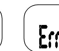
If you do not place the compass correctly while calibrating it, Err appears. If this happens, start over.
